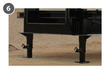
**Dual Drop Foot Jacks** Dual HD drop foot jacks and expanded metal basket are standard on all goosenecks for increased stability, lift and storage capacity.
