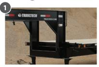
**Step & Grab Handles** Gooseneck step and grab handles make it easier and safer to get up onto the trailer deck.
