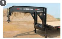
**Drop Gooseneck & Toolbox** The raised height of the gooseneck accomodates newer trucks with higher boxes.
