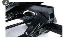
**Scissor Hoist**The heavy duty high lift hoist provides stability, strength, and optimal dumping angle.
