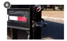
**Hitches**Models are available with either pintle or gooseneck hitches allowing you to match any tow vehicle requirements.
