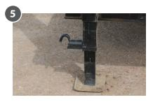
**Dual Drop Foot Jacks**Dual HD drop foot jacks and expanded metal basket are standard on all goosenecks for increased stability, lift and storage capacity.
